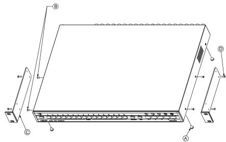
Figure 4. Rack Installation
